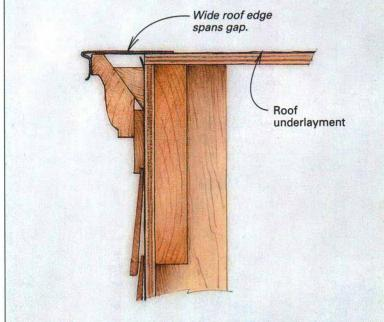
ting into the framing. Any water coming from higher up the wall encountered no weather barrier to direct it out over the metal flashing.
