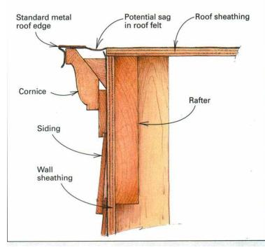
**Wide roof edge spans gap.** Metal roof edge with a 4½-in. flange will span any gap between a cornice detail and the roof sheathing, preventing sag in roof underlayment and shingles and cutting off a possible source of water leaks.
