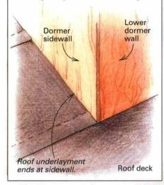
Lap roof underlayment up intersecting walls. A better seal is provided when roof underlayment is lapped 4 in. up any intersecting vertical walls. Follow that with conventional metal step or apron flashing with the shingles.
