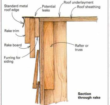
**Keep the seams covered.** Applying metal roof edge that has a wider top flange will keep vertical joints along roof edges covered (left). A better option (drawing right) is to extend roof sheathing far enough to cover the seams. If so, standard metal roof edge would be wide enough.
