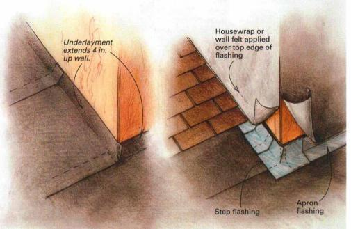
flashing installations, I've found four situations where mistakes commonly occur: around vinylclad and aluminum-clad windows manufactured with nailing flanges, at the intersection of a roof and a sidewall (a dormer, for example), where an outside deck intersects the sidewall of a house and, finally, at the edge of a roof. Correctly flashing these spots won't take much more time than doing it wrong, and the effort will save you lots of heartache.
